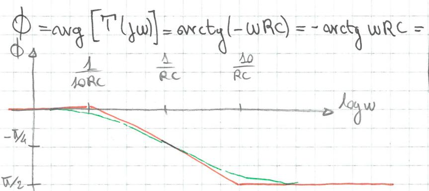
$$\begin{cases} \text{se } \omega \ll \frac{1}{RC} & \phi = 0 \\ \text{se } \omega = \frac{1}{RC} & \phi = -\frac{\pi}{4} \\ \text{se } \omega \gg \frac{1}{RC} & \phi = -\frac{\pi}{2} \end{cases}$$
