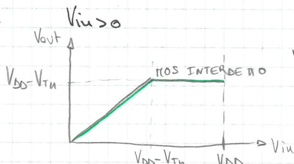
$V_{in} > V_{DD} - V_{TN}$   $V_{out} = V_{DD}$  no canale
