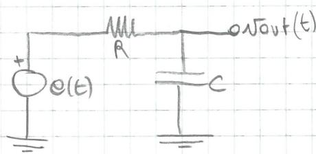
$$e(t) = \sqrt{2} E \sin \omega t \quad Z_R = R \quad Z_C = \frac{1}{j\omega C}$$
